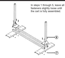
1. Assemble the uprights (3), center brace (2), and caster channels (1).
